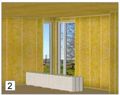
2. The panel boards must be allowed to acclimatise in the packaging at room temperature for 2 days prior to installation.
