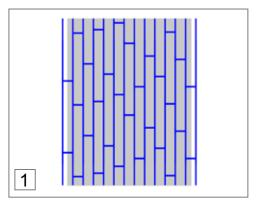
I. Distribute the width so that the first and last panel board are of equal width.
