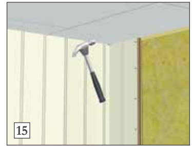
15) Then nail the panel in the fixing lip. In the corner nail the panel visibly with shank nails (hand nailing). Bottom and top can be nailed in the usual way. The correction paint (in the original colour) can be used to paint the heads of the visible shank nails. Apply with the brush in the lid of the correction paint bottle (see picture below).
