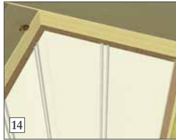
14) Make sure the panel has been thoroughly tapped into place.
