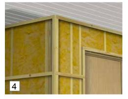
3/4. Install blocking in internal and external corners.
