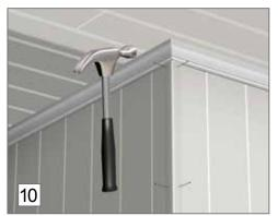
10. Huntonit's corner mouldings can be used for external and internal corners.
