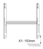
Insert a screw in the lower keyhole approx. 153mm above the floor. Level the bracket and insert the other 3 screws. When the heater is installed, the distance below should be approx. 10 cm.
